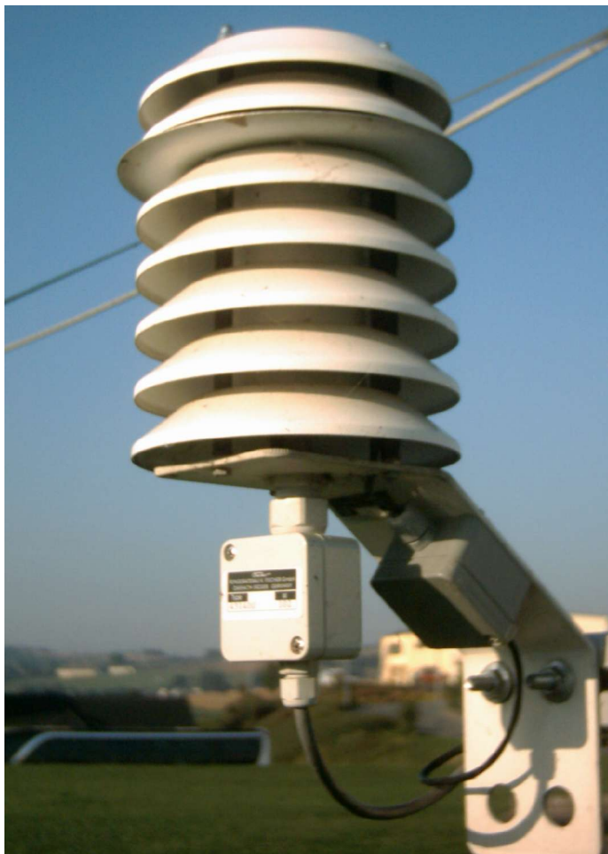
Example: radiation shield 439102 and T/H-sensor 431200
