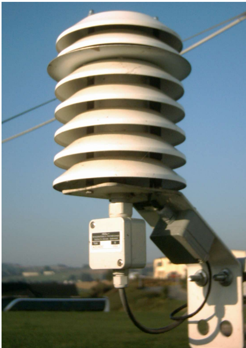
Example: radiation shield 439102 and T/H-sensor 431400
