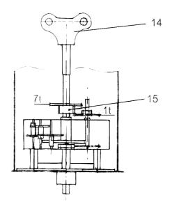
Unscrew the clockwork key (14) in the clockwise direction, present at the drum. Subsequently, you seize the drum (1) with both hands under the edge and take it off upward from the clockwork.
